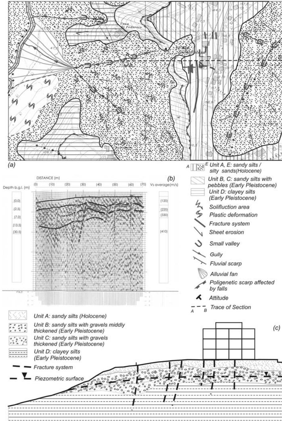
Figure 3. a) geomorphologic map; b) interpretative scheme of the seismic with High-Resolution reflection; c) geological section.
