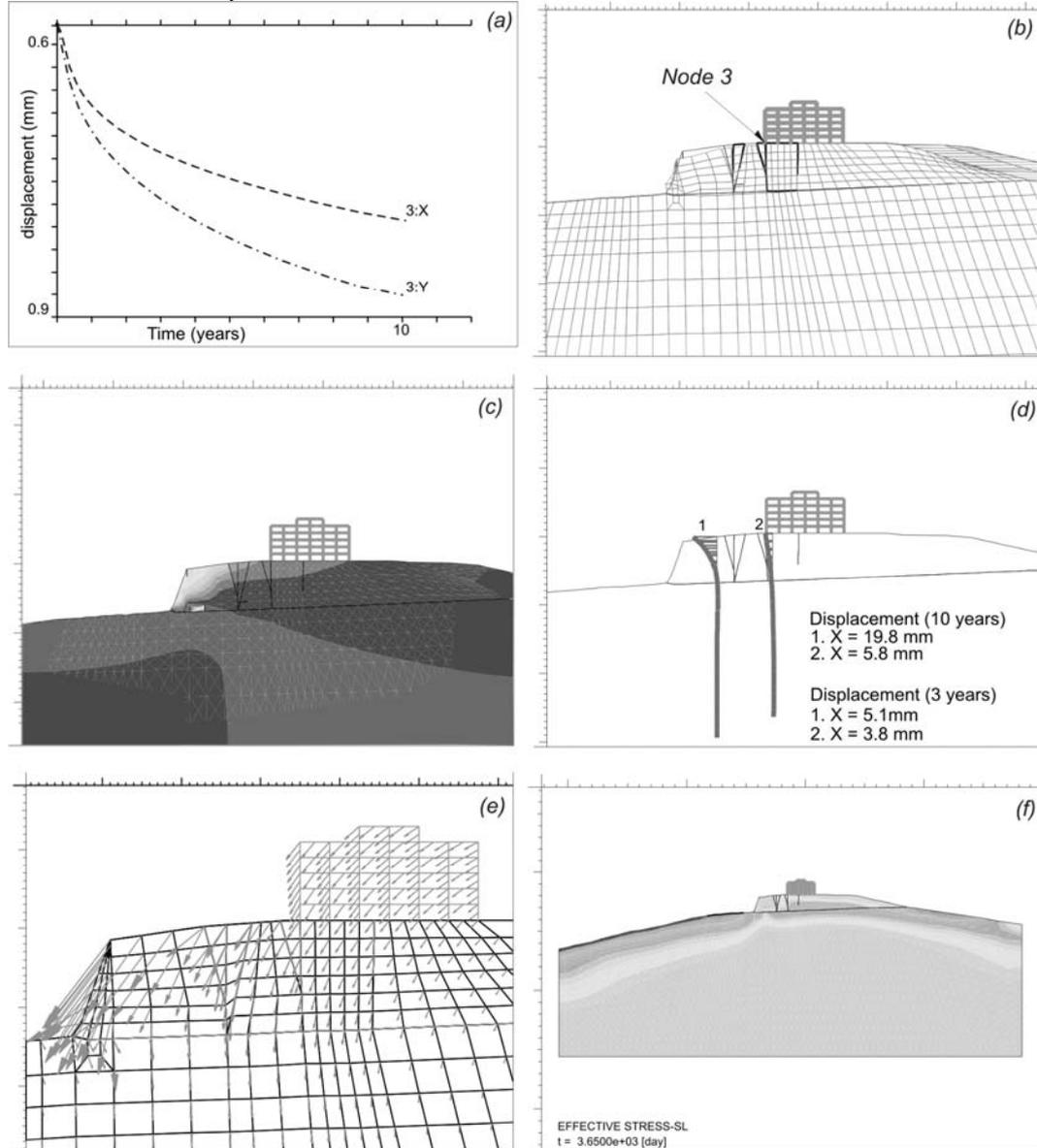
Figure 4. a) time-displacements curves (X → horizontal, Y → vertical) of knot 3; b) deformed mesh; c) horizontal displacements; d) numerical inclinometers; e) displacement vectors; f) effective stress-level.
