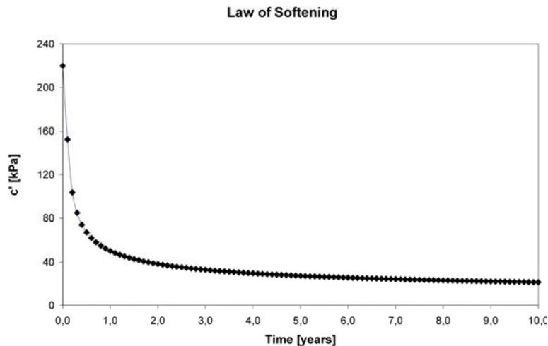
Figure 5. Law of softening deduced through an experimental way .
