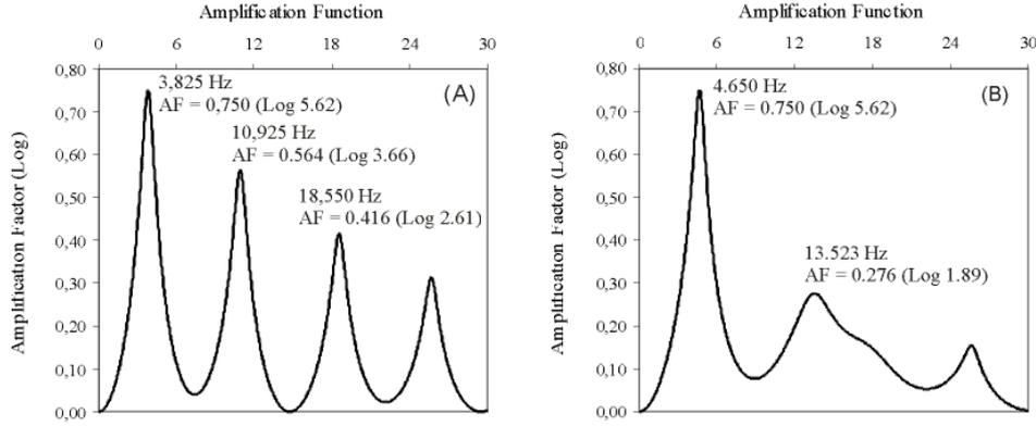
Figure 3. Spectral content of the DAF: A) model 1-D; B) model 2-D.
