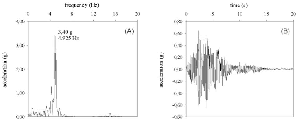
Figure 5. Earthquake to the soil: A) in the frequencies domain; B) in the time domain (IFFT).
