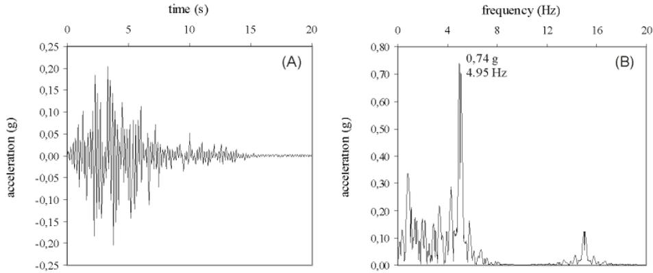
Figure 4. Earthquake project: A) in the domain of time; B) in the domain of frequency (FFT).
