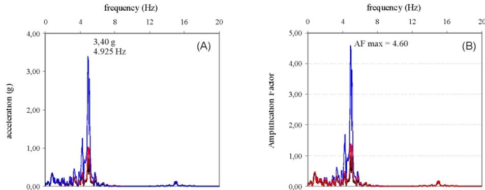
Figure 6: A) Comparison among the acceleration spectra; B) normalized spectra of acceleration.
